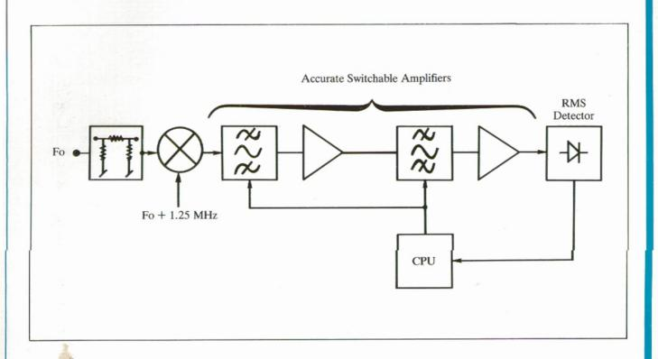
The frequency Fo coming from the attenuator under test enters the attenuation-bridge and is then mixed with the local oscillator frequency Fo  $\pm$  1.25 MHz.
